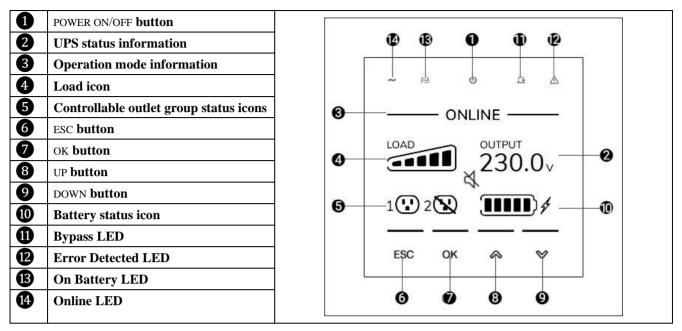
The icons on the LCD display interface screen may vary depending on the installed firmware version.
